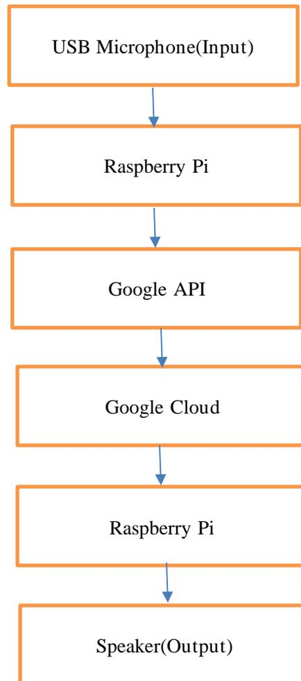
Start to talk to the Google Assistant by saying "Hey Google.". Then input from your voice going through USB Microphone and going to Raspberry Pi and Raspberry Pi send the input to the Google API to recognize your command and voices. Google API send the data to the Google cloud and cloud send the data to the Raspberry Pi to make the output in speaker.
