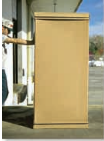
Depending upon where the man pushes on the crate, it will either tip or slip. (© Russell C. Hibbeler)
