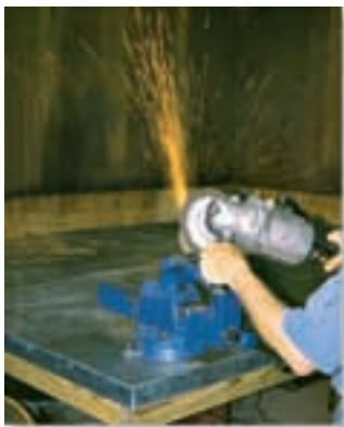
The heat generated by the abrasive action of friction can be noticed when using this grinder to sharpen a metal blade. (© Russell C. Hibbeler)
